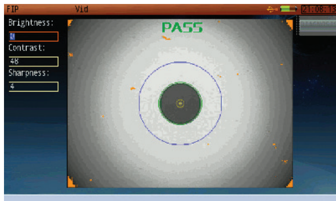
Figure 34: Inspect the face of the fiber optic connectors with the Fiberscope. Pass/Fail software interprets results.
