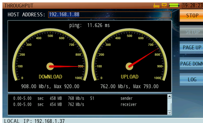
Figure 29: The IP test suite includes tests such as Ping, traceroute and FTP download/upload.
