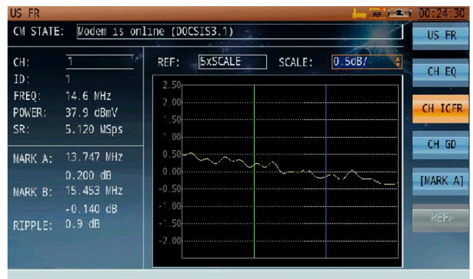
Figure 25: Get Upstream in-channel frequency response from the integrated DS2831 US Cable Modem.
