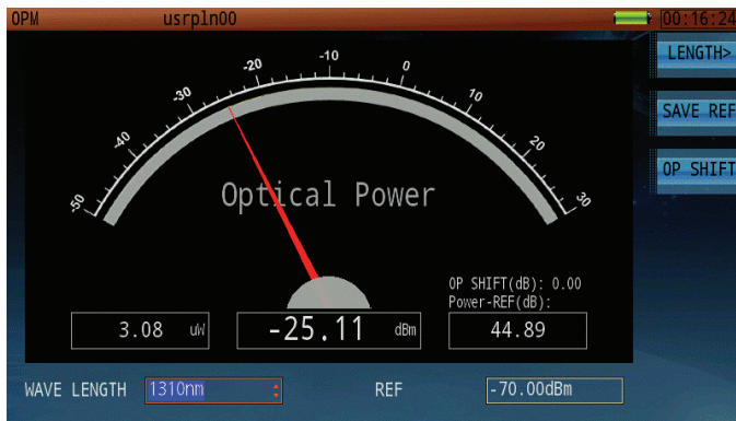
Figure 32: Measure the Optical Power levels at equipment or connector with an easy to interpret graphical gauge.
