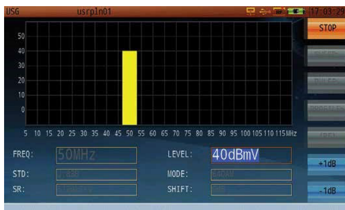
Figure 26: The Upstream Signal Generator can generate C/W carriers to QAM signals.
