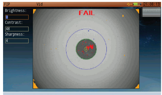
Figure 35: Fiberscope test with dirty connector.
