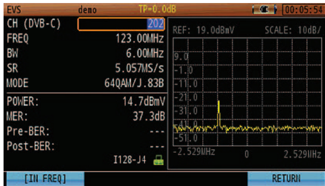
Figure 7: The EVS mode finds narrow-band interference signals with supreme clarity and ease.
