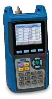
The AE700 is a DWDM Channel Analyzer for the installation and maintenance of DWDM systems. This capable handheld unit measures wavelengths in the C-band ( $1527 \sim 1567$  nm) or L-band ( $1570 \sim 1610$  nm), with additional support for optical signal to ratio (OSNR) - essential for verifying signal quality. Measurements can be displayed in graphical and list formats.
